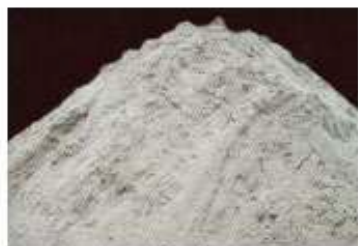
The sand final output contains less than 3% organics and 5% water.
