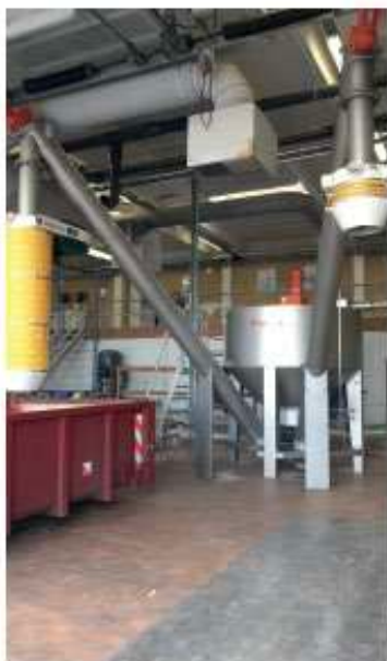
By the addition of a second screw conveyor, the sand output capacity increases to 3 tons/h per sand washer.
